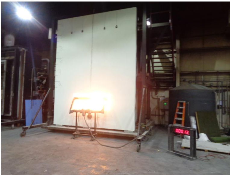
Photo No. 12 Room Burner Ignition
