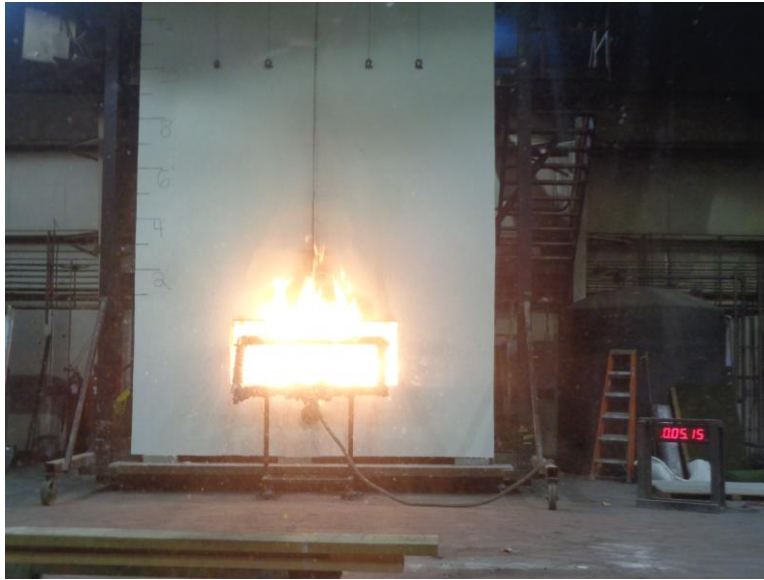
Photo No. 13 Window Burner Ignition
