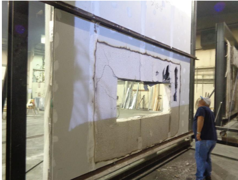
Photo No. 17 First Floor Gypsum (Post-Test)
