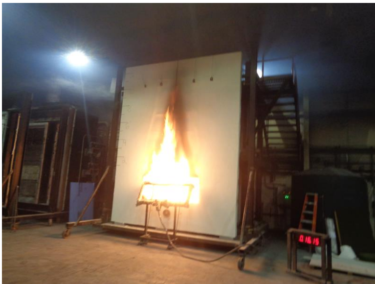
Photo No. 14 Surface Ignition
